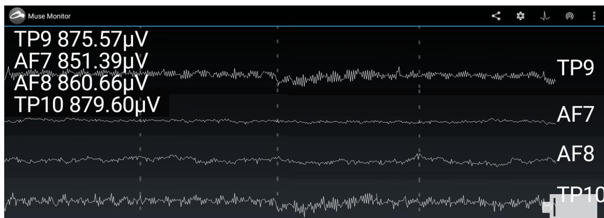
**Figure 1** - The raw voltages recorded at each of the Muse headband's four sensor sites. Time proceeds to the right. Dashed vertical lines mark 1-second intervals.
